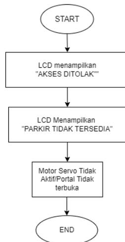
Gambar 4. Diagram Alir Sub-Program *cardRejected*
